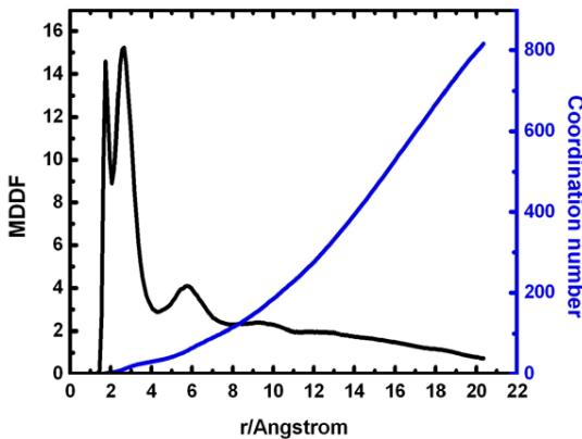
**Fig. 5.** (Color online) Minimum distance distribution function (MDDF) between the smallest distance of all QC atoms and all methanol atoms. The blue bold line corresponds to the coordination number obtained in the MDDF.
